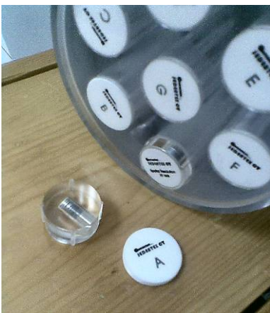
Figure 5: The lettered threaded caps and the orientation rails
